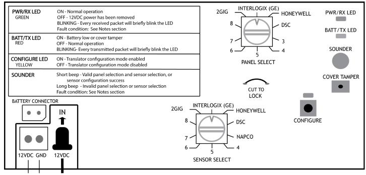
OPTIONAL BARREL CONNECTOR CONNECTOR 12VDC 0.1A 12VDC 1A
