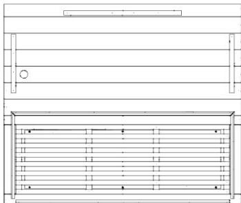
P01 FLOOR PANEL - W2A04760 (x1) 4 5/8"x40 1/16"x47 11/16" (118x1018x1212)
