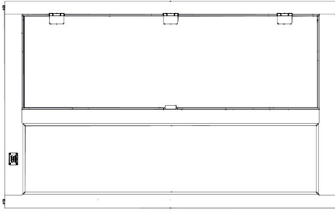
P07 DOOR PANEL - W2A04762 (x1) 1 7/16"x47 11/16"x76 9/16" (36x1212x1944)
