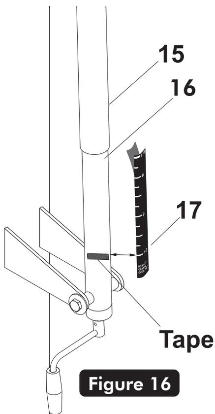
25. Remove the adhesive backing from the Height Decal (#17). Next, carefully align and stick decal to backside of steel actuator (#16) starting at the **10 ft mark first**. Be sure to keep the height decal straight and rub out all air bubbles. See **Figure 16**.
