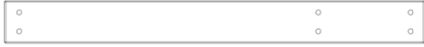
E3 | RAIL DE SOL DU NID DE CORBEAU - W4L12690 (2) | 1 3/8"x3 3/8"x33 1/2" (36x86x852)
