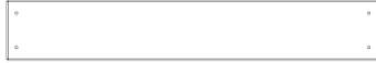
L1 | PLANCHE DE SOL DU NID DE CORBEAU - W4L12742 (6) | 5/8"x4 3/8"x27" (16x112x686)
