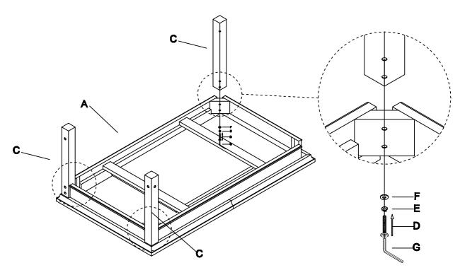
Attach Bottom Shelf (B) to 3pcs Metal Leg (C) using Bolt (D), Spring Washer (E), Flat Washer (F) by Wrench (G), then assemble the 4th Metal Leg (C) on Top Panel (A) and Bottom Shelf (B) by the same method. Finally attach Caster (H) on the Bottom Shelf (B) by using Screw (I).
