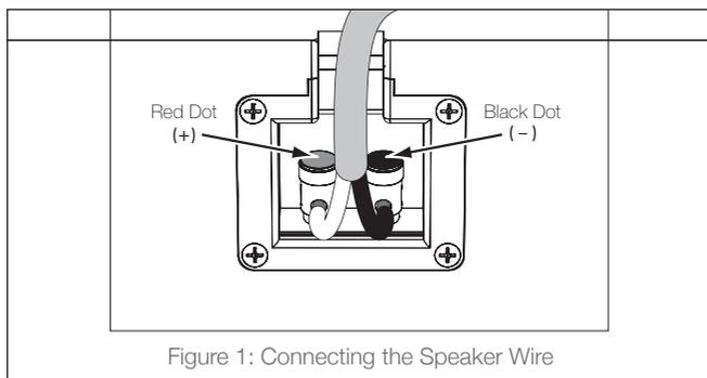
4. The speaker's positive spring terminal is labeled with a red dot; the negative spring terminal is labeled with a black dot.
