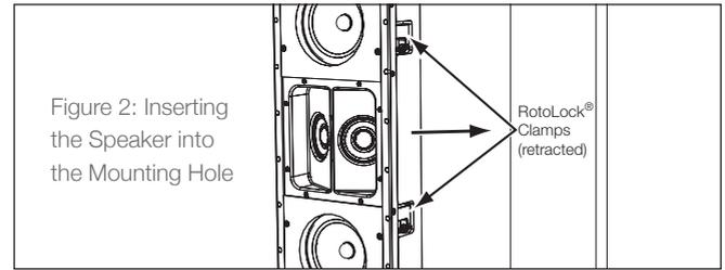
**NOTE: THE ROTOLock® SYSTEM CAN ACCOMMODATE A WALL MATERIAL THICKNESS OF 1 1/4" (32MM). WITH THE TOGGLE FOOT CAP REMOVED, THE SYSTEM CAN ACCOMMODATE A WALL MATERIAL THICKNESS OF 1 1/8" (48MM).**
