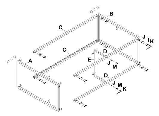
Attach Bottom Drawer (F) to the Left Side Frame (A) and Middle Frame (E) by Bolt (I) and Washer (J) with Allen Wrench (K) as shown.
