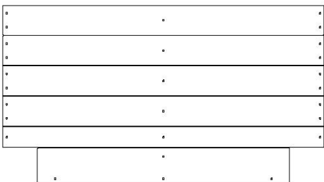
HH1 | PANEL DE PISO - W2A03079 (x2) | 1 1/4"x20 1/8"x36 3/8" (32x510x924)
