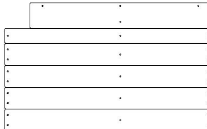
HH6 | PANEL DE PISO - W2A03077 (x1) | 1 1/4"x20 1/8"x32 7/16" (32x510x824)
