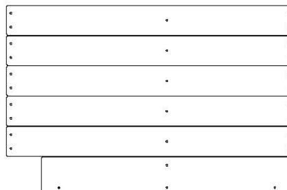
HH4 | PANEL DE PISO - W2A03075 (x1) | 32 7/16"x1 1/4"x21 1/8" (824x32x536)
