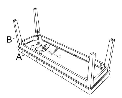
Stand chair up on an even surface and check that it is balanced. If there is a slight wobble, apply downward pressure in the corner where a leg is uneven. Keeping pressure in that corner, tighten all bolts. If balanced,apply downward pressure evenly in the center and tighten all bolts.
