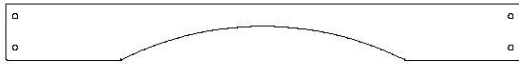
L5 LISSE MURALE DU PAVILLON - W4L14567 (x1) | 5/8 po x 4 3/8 po x 40 3/8 po (16x112x1024)
