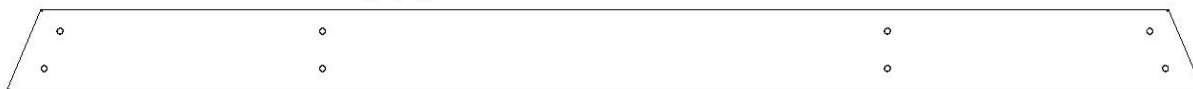
K4 | PLANCHE DE SOL - W4L14560 (x1) | 5/8 po x 5 1/4 po x 78 1/4 po (16x134x1986)
