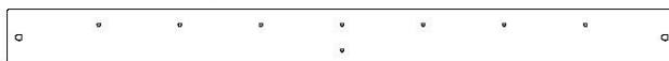
M3 | SUPPORT DE PLANCHER - W4L14573 (x1) | 5/8 po x 3 3/8 po x 40 3/8 po (16x86x1024)
