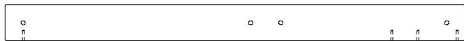
E4 | PIED DU PAVILLON - W4L14534 (x1) | 1 3/8 po x 3 3/8 po x 43 1/8 po (36x86x1094)
