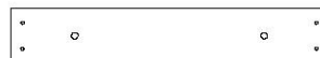
H82 | PLANCHE DE FIXATION - W4L17613 (x1) | 1 po x 3 3/8 po x 19 1/8 po (24x86x486)
