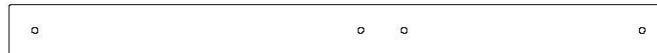
E4 | PIED DU PAVILLON - W4L14534 (x1) | 1 3/8 po x 3 3/8 po x 43 1/8 po (36x86x1094)
