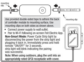
Note: To activate smart features, press and hold the controller module button down for 5 seconds while the unit is off to enter pairing mode. Your unit will cycle through RGB and then pulse a soft white light for 3 minutes. If you need to restart pairing, repeat the process.
