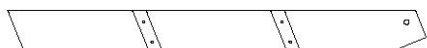
E02 | RAIL D'ÉCHELLE - W4L13970 (x3) | 1 3/8 po x 3 3/8 po x 32 3/4 po (36 x 86 x 831)
