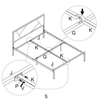
Attach Support Leg (I) to Center Rail (K) using Bolt (Q) with Ratchet Tool (V). Then attach Center Support Leg (H) and Bracket (N) to Center Cross Bar (G) using Bolt (S) and Nut (T) with Ratchet Tool (V) and Wrench (W).
