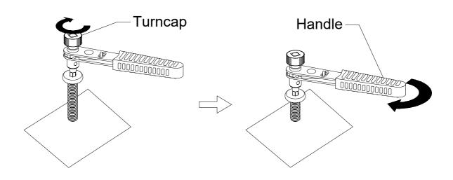
• Loosen bolts: Rotate the handle counterclockwise to loosen the bolt. Then continue rotating the turncap in the same direction to remove the bolt completely.
