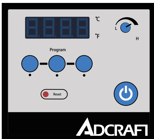
Figure 1. Front of Control Panel
