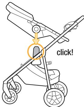
Attach the stroller seat rear-facing or forward-facing to the attachments on the stroller frame.
