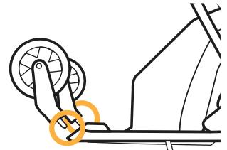
Attach the front swivel wheels as shown.
