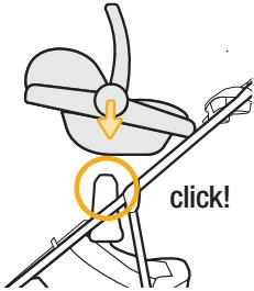
Attach the car seat rear-facing or forward-facing to the attachments on the stroller frame.
