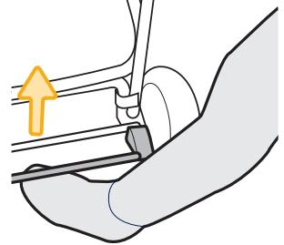
Pull the brake bar up to release.
