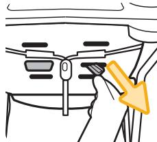
Pull the harness strap retainers through the harness slots.
