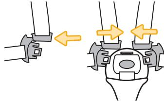
Align the buckle tongue with the tab on top of the buckle. Slide into place.
