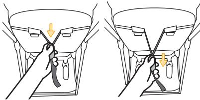
Fully recline the stroller seat backrest. At the back of the stroller seat, press the button on the backrest adjuster all the way and pull it towards you.
