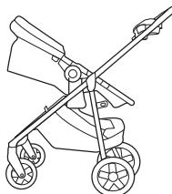
Fold the canopy back. Adjust the stroller seat to the most upright position.
