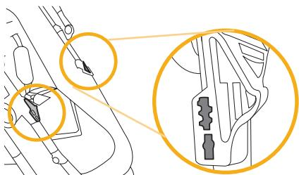
Locate the child tray attachment hubs on each side of the stroller frame.
