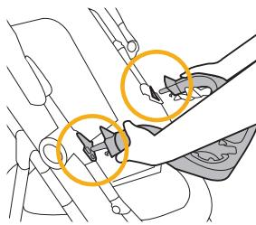
Align the posts on the child tray with the slots in the attachment hubs.
