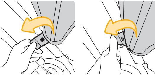
Align the canopy tabs with the attachment on the stroller frame and push the canopy tabs down to snap them to the stroller frame.
