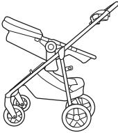
Attach the stroller seat either rear-facing or forward-facing to the attachments on the stroller frame.
