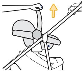
Pull the car seat up either at the carry handle or handle hubs to check if it is attached securely.
