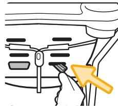
From the back of the stroller seat, push the harness strap retainers through the harness slots.
