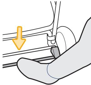
Step on the brake bar to lock.
