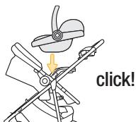
Install the car seat to the attachments on the stroller seat. You will hear each side “click” when it is secure.
