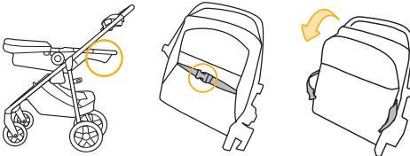
Locate the strap under the footrest. Undo the buckle on the strap as shown.
