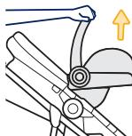
Pull the car seat up either at the carry handle or handle hubs to check if it is attached securely.
