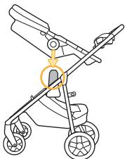
Install the stroller seat either rear-facing or forward-facing to the attachments on the stroller frame. You will hear each side “click” when it is locked into place.
