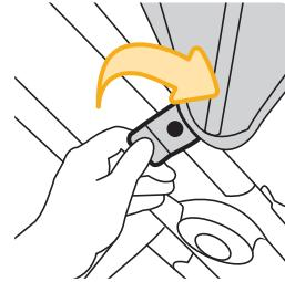
Locate the canopy tabs and pull them forward to remove the canopy from the stroller frame.
