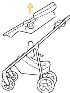
Press the release buttons on each side of the seat all the way in and lift the stroller seat up and off of the stroller frame.
