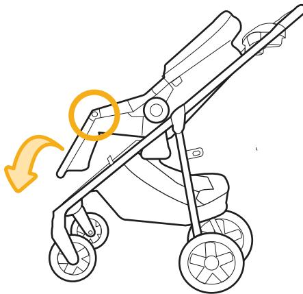
**To lower footrest**, press the footrest adjustment buttons and push down on the footrest.
