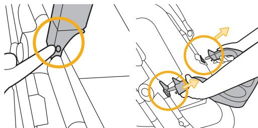
Locate the buttons underneath each side of child tray.
