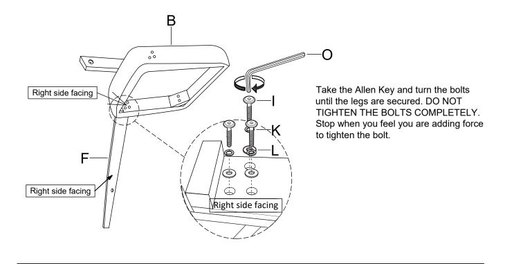
Attach the Left Back Leg (E) to the Cushion Seat (B) using JCBC Bolt (I), Lock Washer (K) and Flat Washer (L) with the Allen Key (O).
