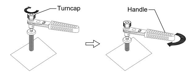
• Loosen bolts: Rotate the handle counterclockwise to loosen the bolt. Then continue rotating the turncap in the same direction to remove the bolt completely.
