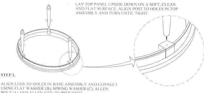
USING FLAT WASHER (B), SPRING WASHER (C), ALLEN BOLT (A) AND ALLEN KEY (D) PROVIDED.
