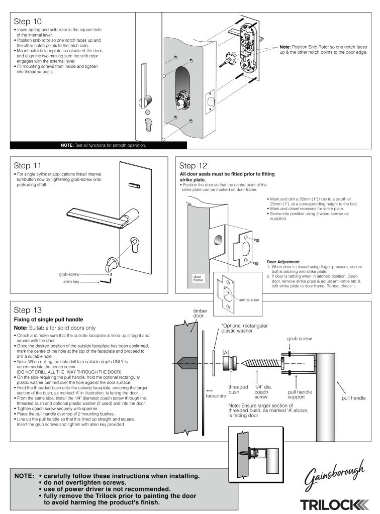
Single Pull Handle Version - Suits 35mm to 45mm door thickness
