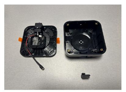
4. Place the Rubber Grommet around the 24V Power Supply cable with the hook of the grommet facing towards the barrel connector.
