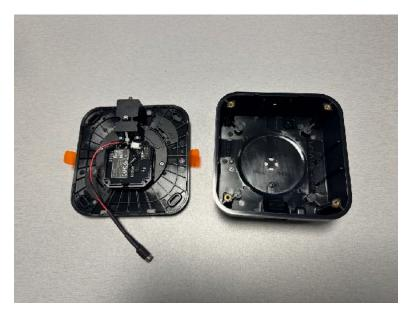
3. Remove the rubber grommet from the bottom of the VESA Station
