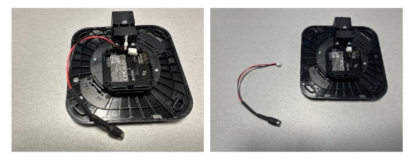
5. Remove the Blue phoenix connector, 2 small screws and phoenix connector from the power supply box.
