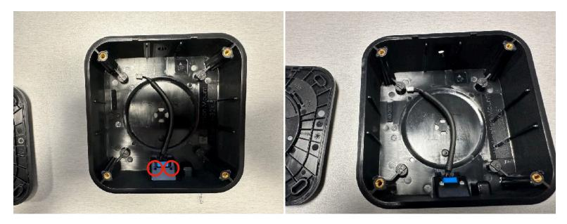
9. Attach the White Molex connector onto the VESA Station board making sure the securely seat the connector before finishing installation.
