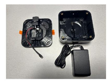
6. Attach the barrel connector to the VESA station and install the provided screws to secure the station to the mounting box.
