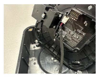
10. Install the provided screws to secure the station to the mounting box remembering to fist remove the VESA Station Cover. Now attached the VESA Station using 2 wire cable to the vehicles Positive and Ground 12-24V system.
