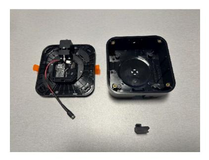
4. Cut the zip tie holding the DC barrel connector into place and remove the cable.
