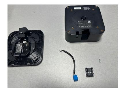
6. Attach the Phoenix connector cover on the the blue phoenix connector making sure the holes line up with the connector and the cover.
