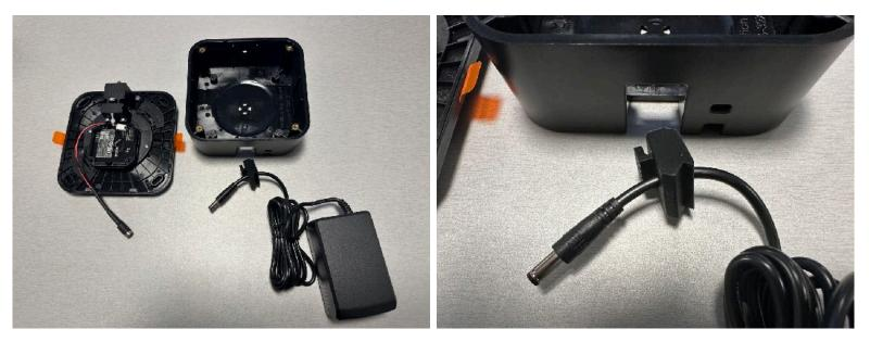
5. Reinstall the grommet and barrel connector through the VESA Station making sure to fully seat the grommet back into place.
