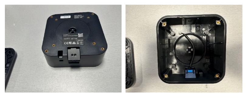
8. Secure the Phoenix cover with the two small Philips screws.
