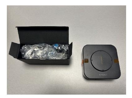
2. Remove the orange adhesive tabs holding the VESA Station together and separate the two halves.
