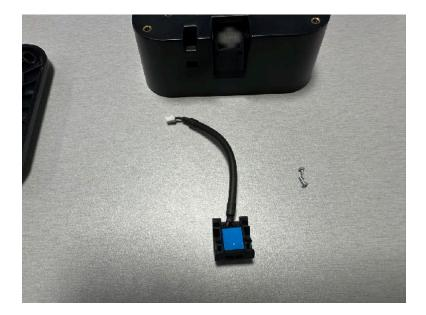
7. Place the Cable into the VESA Mount and turn the mount face up.
