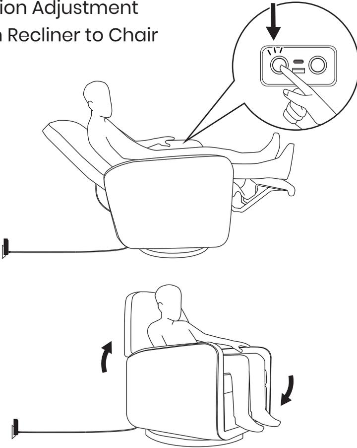
The chair is returned to the upright position by pressing the button located at the inside right of the armrest.
