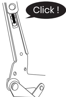
Firmly push each side into place one at a time. **You should hear a click** when the chair back locks into place on each side.
