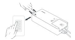
2. Very quickly, click and release the "Learn" button and, within 5 seconds, quickly click and release one of the "Up Arrow" buttons on the Controller for any of the Zones. When lights blink, Controller and Receiver are paired. Repeat process until Zones are paired as desired.
