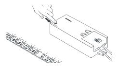
1. When pairing additional Zones to the same Controller, clear the memory on the new Receiver for the next Zone by pressing and holding the "Learn" button until the lights blink.
