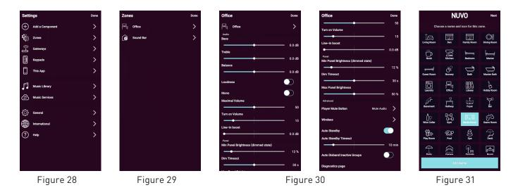
The ZONE SETTINGS screen contains simple slider adjustments or on/off choices that control the sound for the selected zone.
