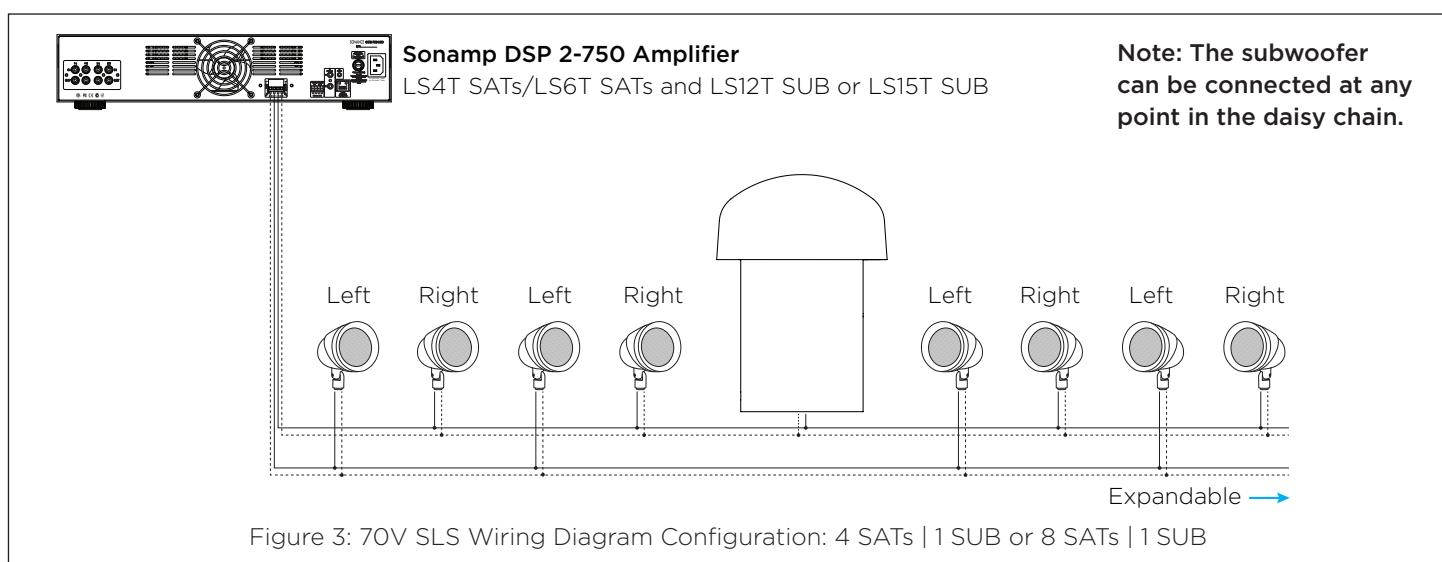
Figure 3: 70V SLS Wiring Diagram Configuration: 4 SATs | 1 SUB or 8 SATs | 1 SUB
