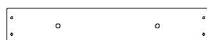
H16 | PLANCHE DE FIXATION - W4L16846 (x2) | 1 po x 3 3/8 po x 19 1/4 po (24x86x488)
