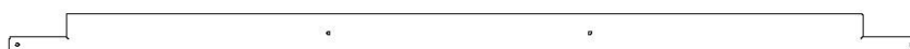
N7 | PLANCHE DE PLANCHER - W4L06457 (x1) | 5/8 po x 2 3/8 po x 54 1/4 po (16x60x1379)
