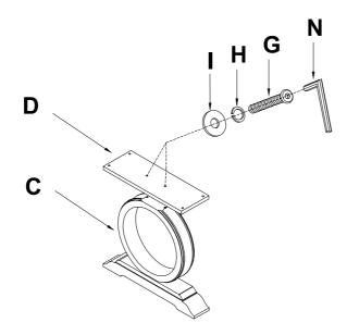
Place the Table Top(A) upside down smooth carpet surface. Tighten the Mounting Plate(D) and Table Top(A) by Bolts(J), Lock Washers(L) and Flat Washers(M) with Allen Wrench(N). Tighten the Center Stretcher(E) and Table Top(A) by Bolts(K), Lock Washers(L) and Flat Washers(M) with Allen Wrench(N). Tighten the Post(C) and Center Cross Bar(F) by Bolts(G), Lock Washers(H) and Flat Washers(I) with Allen Wrench(N).
