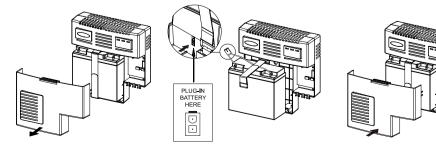
Step 1: a. Remove the battery cover
