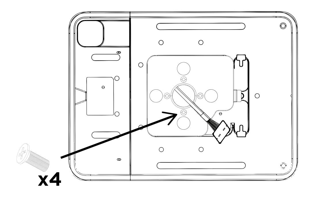
17. Plug the Molex connector from the Mount into the cable on the CONNECT Case. Note that the gold pins face outward when connecting to the Mount cable. Press the Mount cable into the channel to hold and secure the cases in place.
