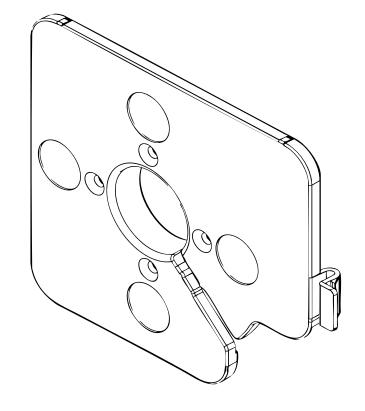
2. Remove the VESA mouting plate from the VESA box and remove the packaged hardware from inside.
