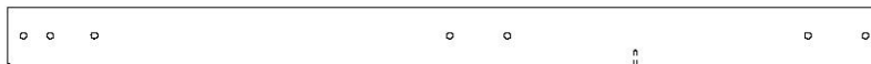
E10 | MONTANT DU FORT - W4L16899 (x1) | 1 3/8 po x 3 3/8 po x 51 3/8 po (36x86x1305)
