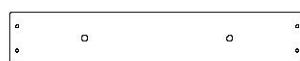
H16 | PLANCHE DE FIXATION - W4L16846 (x2) | 1 po x 3 3/8 po x 19 1/4 po (24x86x488)
