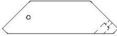
E6 | CALE DE LA PLATEFORME - W4L16834 (x8) | 1 3/8 po x 3 3/8 po x 11 15/16 po (36x86x303)
