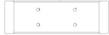
H08 SUPPORT DE CHEVRON - W4L17530 (x1) 15/16 po x 3 3/8 po x 10 11/16 po (24x86x272)
