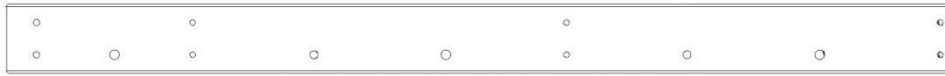
H20 SUPPORT DE CHEVRON - W4L17549 (x1) 15/16 po x 3 3/8 po x 46 3/8 po (24x86x1177)
