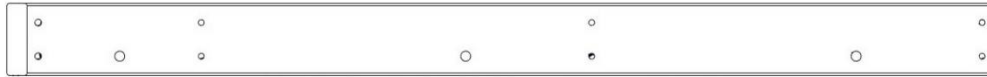
H30 SUPPORT DE CHEVRON - W4L17570 (x1) 15/16 po x 3 3/8 po x 46 3/8 po (24x86x1177)
