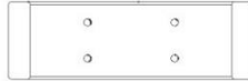
H08 SUPPORT DE CHEVRON - W4L17530 (x2) 15/16 po x 3 3/8 po x 10 11/16 po (24x86x272)
