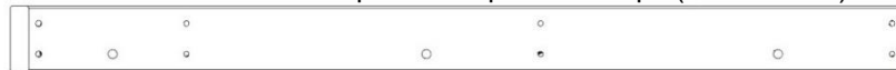
H30 SUPPORT DE CHEVRON - W4L17570 (x2) 15/16 po x 3 3/8 po x 46 3/8 po (24x86x1177)
