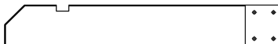
D07 | SOLIVE INTÉRIEURE COURTE - W4L16763 (x6) | 1 7/16 po x 5 1/4 po x 35 1/4 po (36x134x896)
