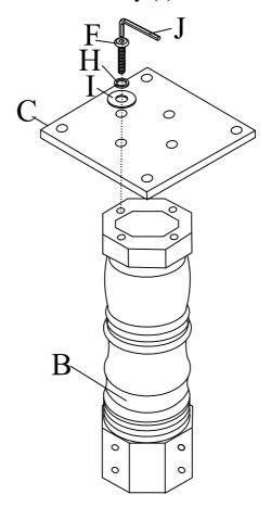
Attach the Mounting Plate (C) to Table Top (A) with Flat Washer (I), Lock Washer (H), Bolt (E) and fully tighten with Allen Key (J). Do not over tighten.
