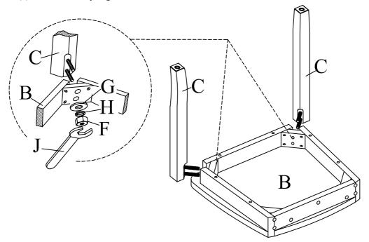
Take the Allen Wrench, and turn the bolts until the legs are secure. DO NOT TIGHTEN COMPLETELY.
