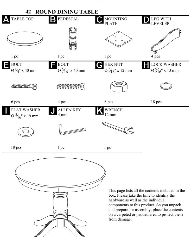
Attach the Mounting Plate (C) to Pedestal (B) with Flat Washer (I), Lock Washer (H), Bolt (F) and fully tighten with Allen Key (J). Do not over tighten.
