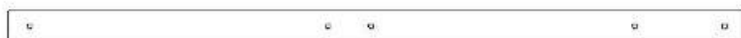
F2 | MONTANT MURAL - W4L12405 (x2) | 1 3/8 po x 2 3/8 po x 57 3/4 po (36 x 60 x 1 467)
