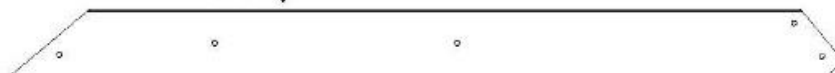
G13 | SUPPORT TRANSVERSAL - W4L12314 (x1) | 1 po x 5 1/4 po x 65 1/4 po (24 x 134 x 1 658)
