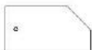
G15 | SUPPORT DE COMPTOIR - W4L12425 (x1) | 1 po x 5 1/4 po x 9 7/8 po (24 x 134 x 250)
