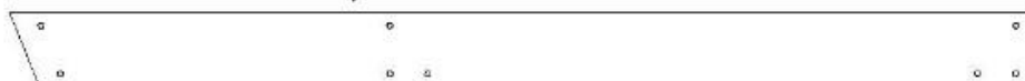
G4 | PLANCHE DE SOL - W4L12293 (x1) | 1 po x 5 1/4 po x 72 1/4 po (24 x 134 x 1 835)
