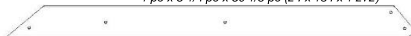
G12 | SUPPORT TRANSVERSAL - W4L12315 (x1) | 1 po x 5 1/4 po x 65 1/4 po (24 x 134 x 1 658)
