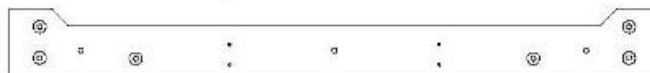
G7 | RAIL DE PLATEFORME - W4L12296 (x1) | 1 po x 5 1/4 po x 51 po (24 x 134 x 1 296)
