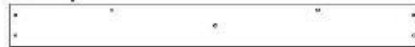
M1 | PLANCHE DE PLATEFORME - W4L12409 (x1) 5/8 po x 3 3/8 po x 32 1/4 o (16 x 86 x 820)
