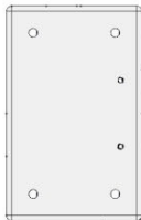
K04 BLOC DE VERROUILLAGE - W4L19789 (x2) 5/8"x3"x4 3/4" (16x76x120)
