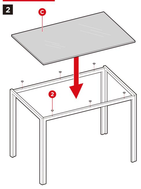
Insert six part 2 suction cups into the assembled frame. Place the part C glass tabletop onto the frame.
