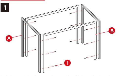
Attach the two part A short table frames to the two part B long tables frames with twelve part 1 screws.
