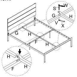
Attach the Support Leg (J) to Center Rail (H), insert the Bolt (P), turn the Ratchet Tool (W) to tighten them. Attach the Center Support Leg (I) and Bracket (O) to Center Cross Bar (F), insert the Bolt (S) and Nut (V), turn the Ratchet Tool (W) and Wrench (X) to tighten them.
