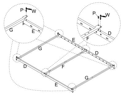
Attach the Center Support Leg (I) to Center Cross Bar (F), insert the Bolt (P), turn the Ratchet Tool (W) to tighten them.
