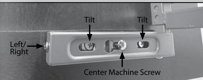
**Left/Right:** Loosen center machine screw and adjust machine screw on side of horizontal door arm. Retighten center screw.
