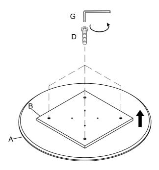
Attach Connecting Panel (B) to Base (C) using Bolt (D), Spring Washer (E) and Flat Washer (F) with Allen Key (G).
