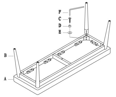
Take the Allen Key, and turn the bolts until the legs are secure. DO NOT TIGHTEN COMPLETELY. Stop when you feel you are adding force to tighten the bolt.
