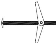
**Toggle Bolt** - Drill hole through wall. Hole must be large enough for the wings to pass through. Insert screw through the holes in the mounting bracket and thread the toggle wings just onto the screw. Fold the wings back and push through the hole until the wings spring open. Pull back on the screw to hold wings against the inside of the wall and tighten screw.
