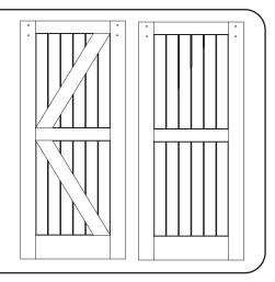
Before drilling the 4 (four) holes for the sliding wheel hardware, ensure your door is positioned correctly with the top and bottom rails properly oriented. The bottom rail is wider, measuring 8 inches, while the top rail is narrower at 4-1/4 inches. It is crucial to drill the holes only into the top rail, following the appropriate measurements as per next figure.
