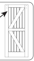
Your door DOES NOT come pre-drilled. To install the two sliding wheels, you will need to drill four (4) holes yourself using a drill and a 3/8" diameter drill bit. Please ensure you maintain the precise distances between the holes.
