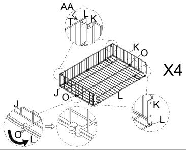
Insert Caster (M) into the Slot of Drawer Bottom Frame (L) and assemble them using Bolt (T) with L-Allen Key (AA).
