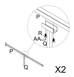
Attach Center Rail (P) to Support Leg (Q). Then attach the assembled part to Center Support Bar (E) using Bolt (S) and Nut (Y) with L-Allen Key (AA) and Wrench (AB).
