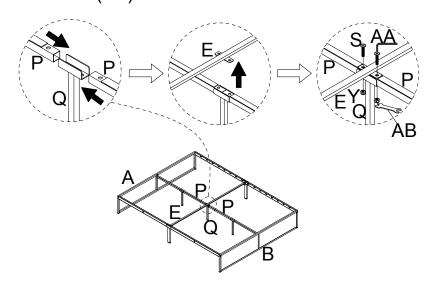
Attach Center Rail (P) to Headboard (A) and Footboard (B) using Bolt (R) with L-Allen Key (AA).
