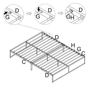
Hook Drawer Left & Right Side Frame (J & K) to Drawer Bottom Frame (L) and assemble them using Bolt (T) with L-Allen Key (AA). Then lock Drawer Frame Connector (O) as shown.
