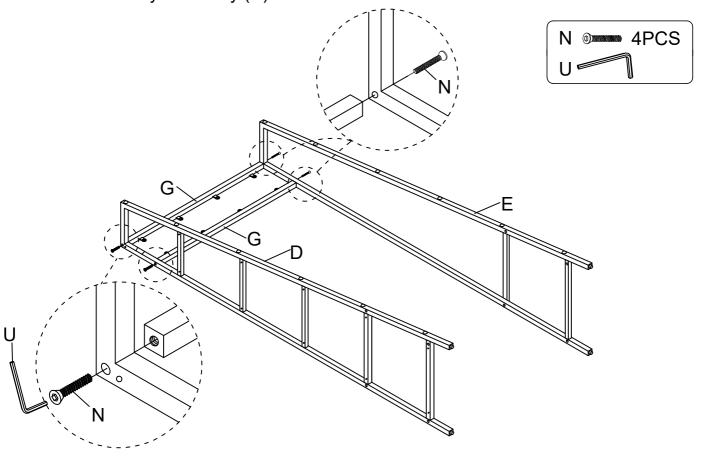
Assemble Top Shelf Panel (A) to the Middle Frame (D) and Right Frame (E) with Bolt (N), then fasten by Allen Key (U).
