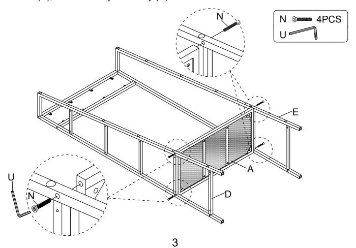
Assemble Bottom Shelf Panel (B) to the Middle Frame (D) and Right Frame (E) with Bolt (N), then fasten by Allen Key (U).
