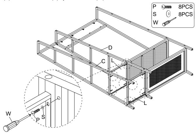
Assemble Shelf Panel (I), Shelf Panel (J), Shelf Panel (K) to the Middle Frame (D) and Left Frame (C) with Bolt (P) and Flat Washer (S) by Screwdriver (W).
