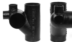
Part No. NH 458 Vented Closet Tee with 2" Top Vent and 2" Side Inlet (Left Hand or Right Hand; Designed for use below the floor; Fitting does not require a baffle.)
