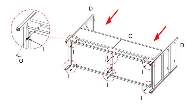
Attach Center Frame (E) to the Drawer (C) by using Bolt (J) and Allen Wrench (O) as shown.
