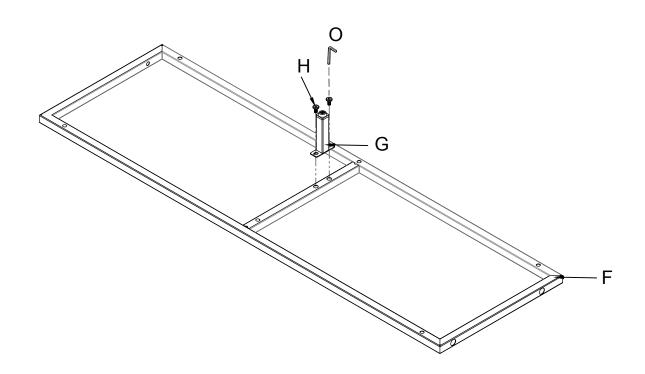
2 Attach Side Frame (D) to the Lower Frame (F) by using Bolt (I) and Allen Wrench (O) as shown.
