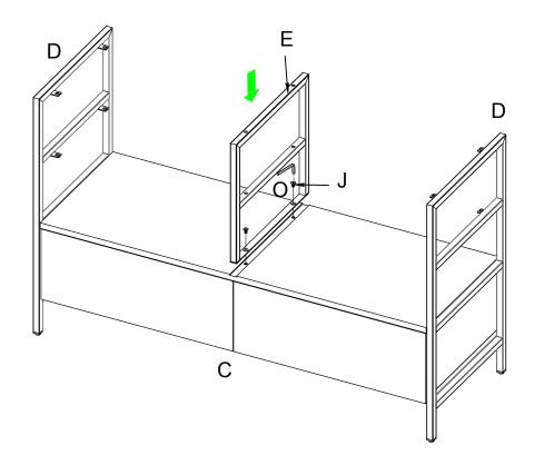
5 Attach Lower Panel (B) to the Side Frame (D) and Center Frame (E) by using Bolt (H), Bolt (I) and Allen Wrench (O) as shown.
