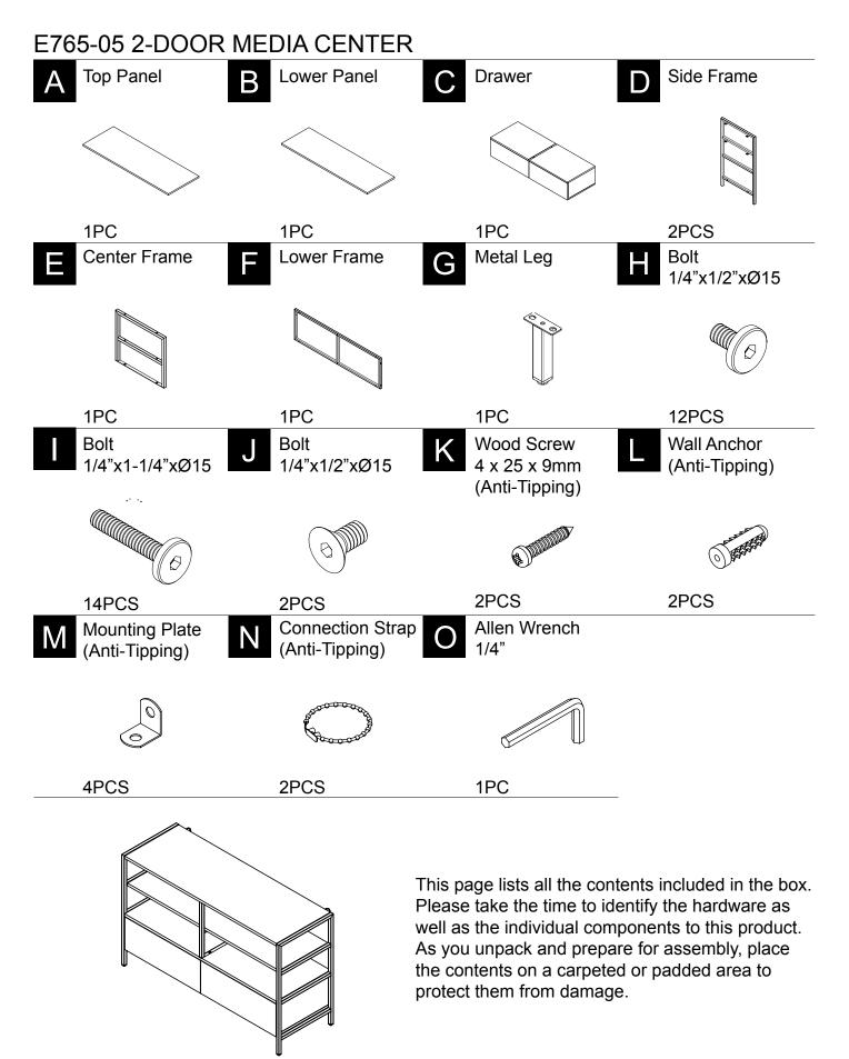
\*\*\*Do not tighten screws & bolts until the entire unit is completely assembled.
