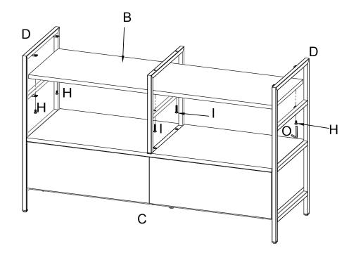
6 Attach Top Panel (A) to the Side Frame (D) and Center Frame (E) by using Bolt (H), Bolt (I) and Allen Wrench (O) as shown.
