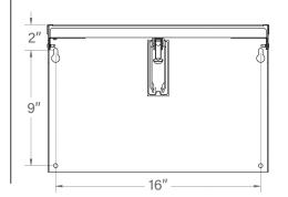
Secure two 1/4" lag bolts or screws (hardware not provided) through upper keyholes of back plate.
