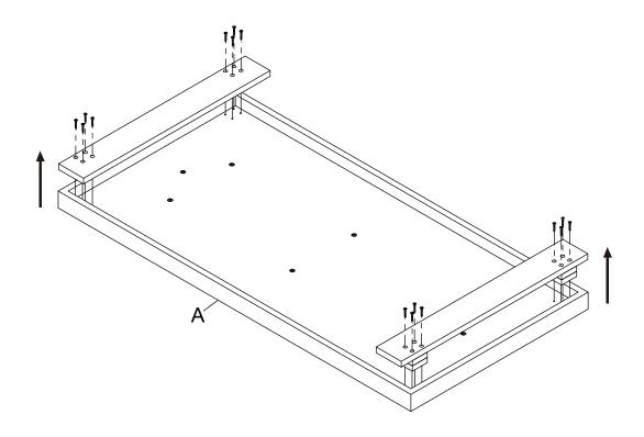
Attach both Side Frames (C) to Upper Cross Bars (D) and Lower Cross Bars (E) using Bolts (H) and Allen Wrench (I) as shown.
