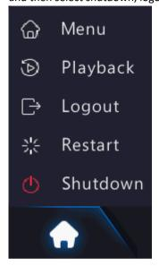
Front panel: Press and hold the power button on the front panel (if available) for 3 seconds until you hear a beep, then hold for 2 seconds until an on-screen message appears, and then click Yes to shut down the
