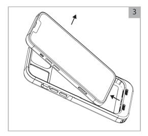
Press the top of the iPhone from behind the case outward enough to clear the edge of the case then pull the iPhone up and out of the case.
