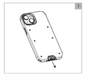
To uninstall the iPhone first remove the Lightning Dongle by sliding it out from the bottom of the Case.
