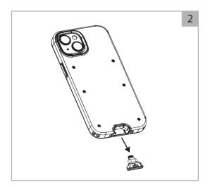
Make sure to completely remove the Lightning Dongle before attempting to remove the iPhone from the Case.
