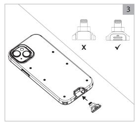
Rotate the case face down and insert the Lightning Dongle (B) into the bottom of the Phone Case (A) making sure to fully seat the Dongle into the Case.
