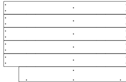
HH4 | FLOOR PANEL - W2A03075 (x1) | 32 7/16"x1 1/4"x21 1/8" (824x32x536)
