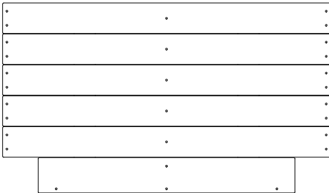
HH3 | FLOOR PANEL - W2A03078 (x2) | 36 3/8"x1 1/4"x21 1/8" (924x32x536)
